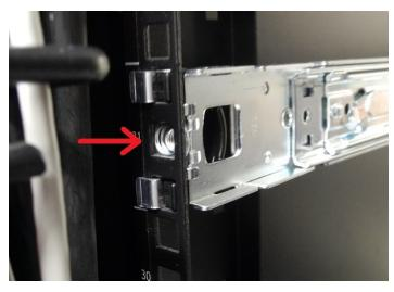
4. Fasten the transformer bracket to each sliding mount with two wide flat-headed screws.
