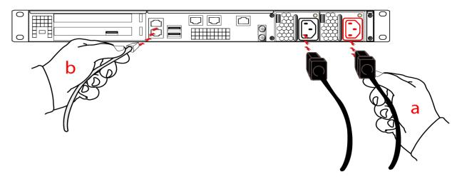
If you have a PED-authenticated SafeNet Luna Network HSM, connect the PED directly to the HSM card's USB port (on the rear panel's left side), using the included USB-to-MiniUSB PED cable. See also "Local PED Setup" on page 1 in the Administration Guide. If you have a password-authenticated HSM, skip to the next step.
