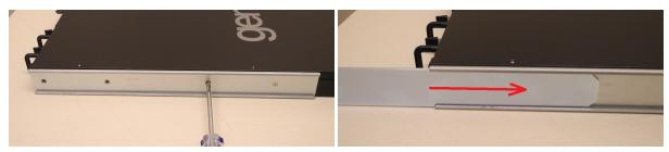
4. Install the two sliding rear brackets in your equipment rack using four rack mounting screws.
