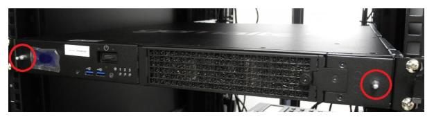
Turn the keys to the vertical position to lock the bezel. The keys cannot be removed if the bezel is unlocked. The two locks are keyed differently, so the keys can be issued to different security personnel and kept in secure, separate locations.
