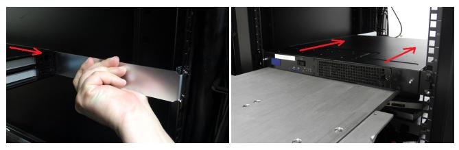
**CAUTION!** Support the weight of the appliance with the hydraulic lift until all four brackets are secured.
